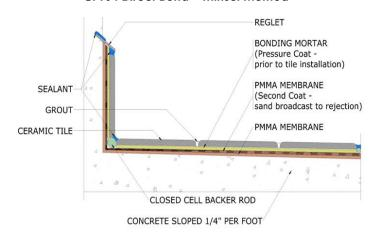
CF101 Bonded Mortar Bed - Thickset Method
