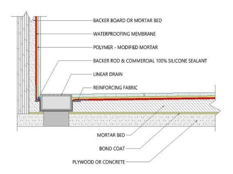
NOTE: Illustrations shows the necessary components of the tile installation method, including the substrate. This has not been drawn to scale.
