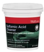
Read entire label before using. Concrete and grout should be cured a minimum of 10 days and be clean. Saturate unglazed tile, concrete, masonry or grout with clean water for one hour prior to application. Apply solution to wet surface and scrub with a nylon bristle brush. Work in small areas. Flush with water immediately after brushing. Do not use repeatedly or surface damage could occur. For heavy concrete etching, allow solution to sit for up to 30 minutes prior to flushing with clean water.
