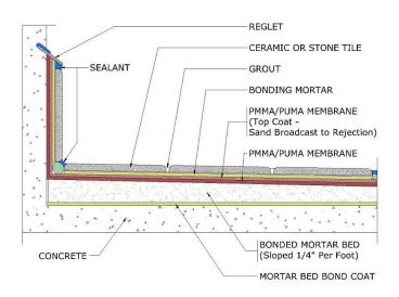
When using any membranes in exterior tile or natural stone applications, attention to the substrate's flatness and providing adequate pitch is required to properly evacuate water. Divots in the plane, commonly referred to as "birdbaths," will trap water leading to expansive efflorescence and/or tile delamination from the effects of thermal growth and freeze-thaw expansion.
