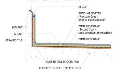
CF101 Bonded Mortar Bed - Thickset Method
