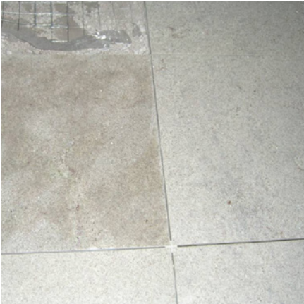
Photo 6: Mock-up Test Showing Sealed Stones vs. an Untreated Piece
